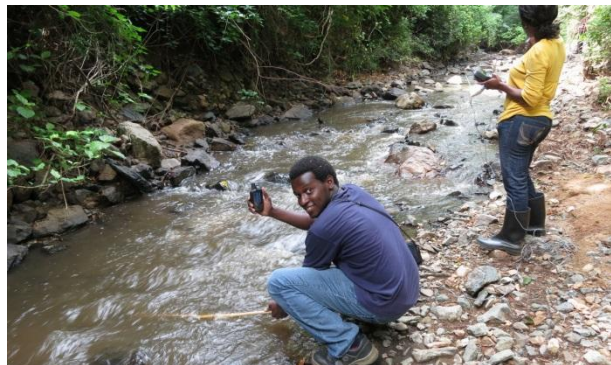
Fig.1: Field Data Collection (Here: measuring the water flow to estimate the hydropower potential of a river).
